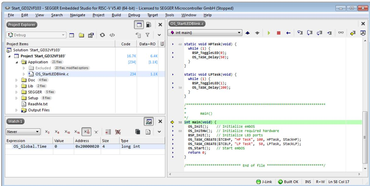
Before you step into `OS_Start()`, you should set two breakpoints in the two tasks as shown below.
