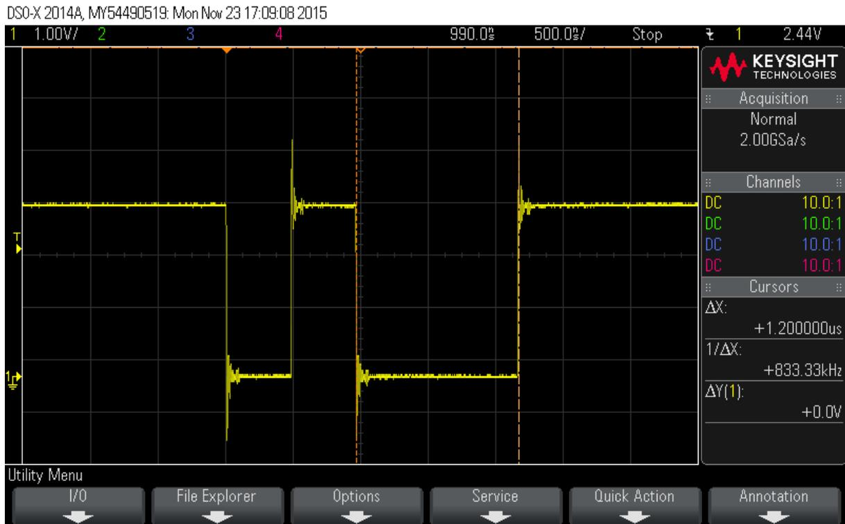
$t_{CD}$  is measured as 12000ns.
