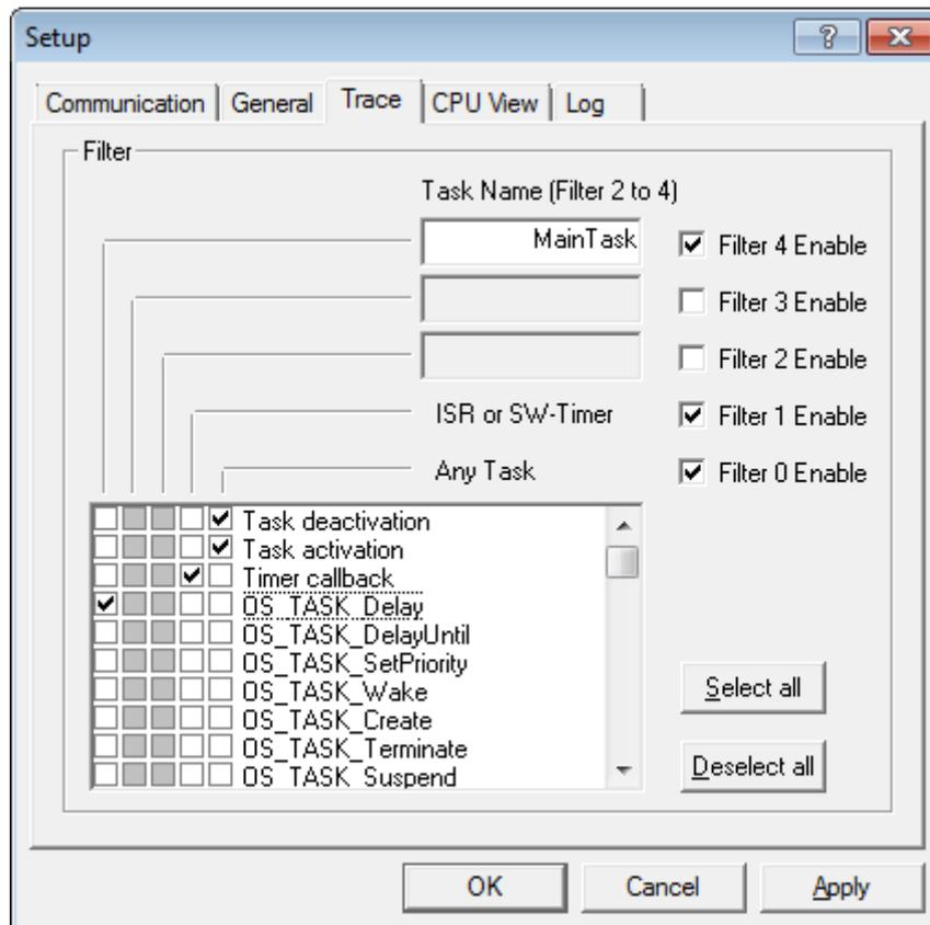
To enable or disable a filter, simply check or uncheck the corresponding checkboxes labeled Filter 4 Enable to Filter 0 Enable. For any of these five filters, individual API functions can be enabled or disabled by checking or unchecking the corresponding checkboxes in the list. To speed up the process, there are two buttons available:
