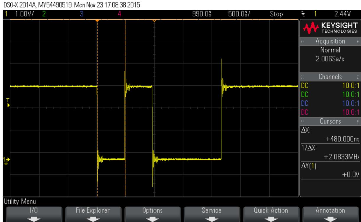
$t_{\text{AB}}$  is measured as 480ns.
