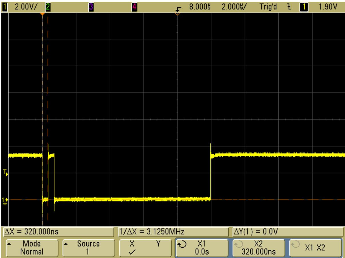
The screenshot below shows the context switch time. The period between the second falling edge and the second rising edge is the context switch time and includes the measurement overhead which has to be subtracted. The measured value is  $T_2 = 9.24 \text{ us}$ .
