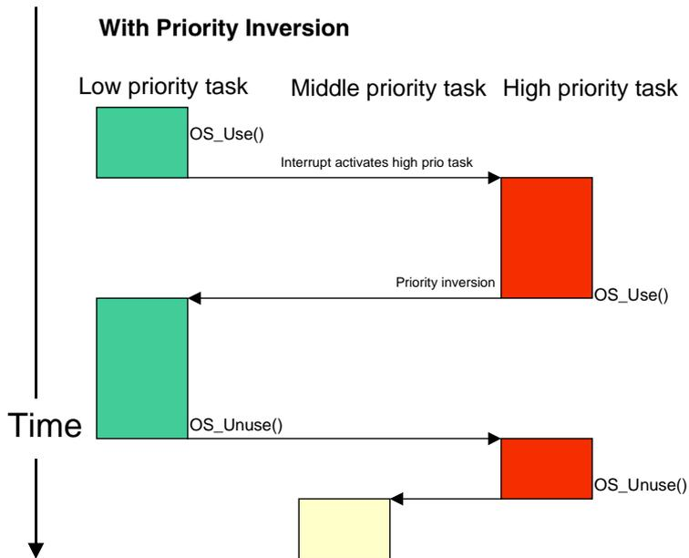
With priority inversion the low priority task is activated instead of the middle priority task when the high priority task tries to claim the semaphore.
