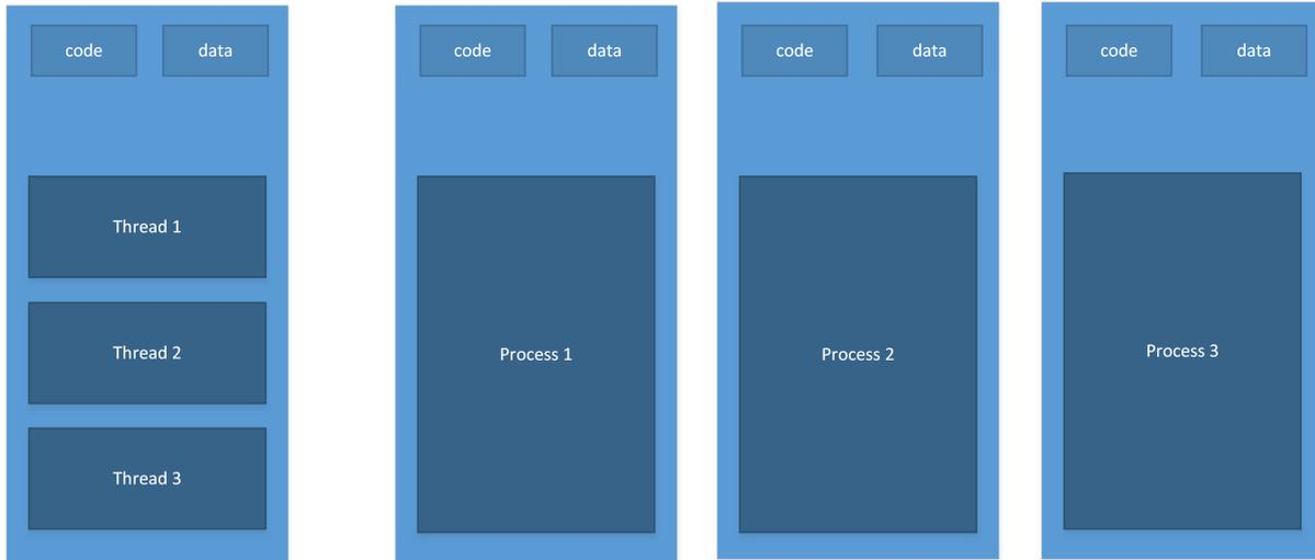
Threads are tasks that share the same memory layout, hence any two threads can access the same memory locations. If virtual memory is used, the same virtual to physical translation and access rights are used.
