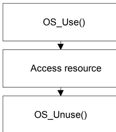
A resource semaphore contains a counter that keeps track of how many times the resource has been claimed by calling `OS_Request()` or `OS_Use()` by a particular task. It is released when that counter reaches zero, which means the `OS_Unuse()` routine must be called exactly the same number of times as `OS_Use()` or `OS_Request()`. If it is not, the resource remains blocked for other tasks.
