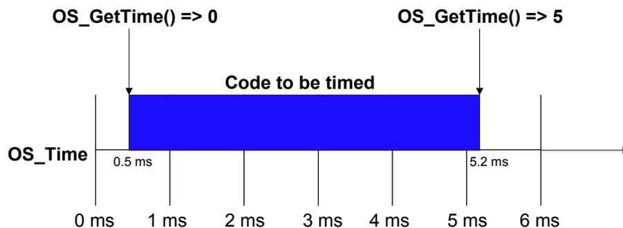
For many applications, low-resolution measurement may be sufficient for your needs. In some cases, it may be more desirable than high-resolution measurement due to its ease of use and faster computation time.
