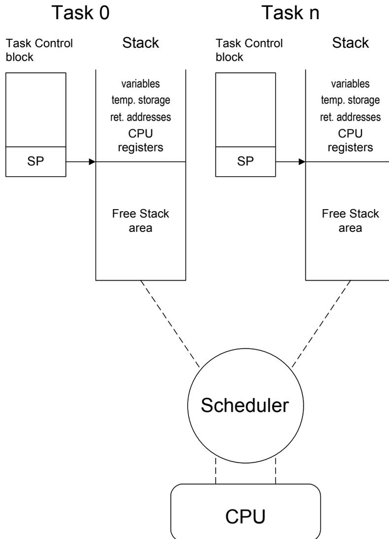
The scheduler deactivates the task to be suspended (Task 0) by saving the processor registers on its stack. It then activates the higher-priority task (Task n) by loading the stack pointer (SP) and the processor registers from the values stored on Task n's stack.
