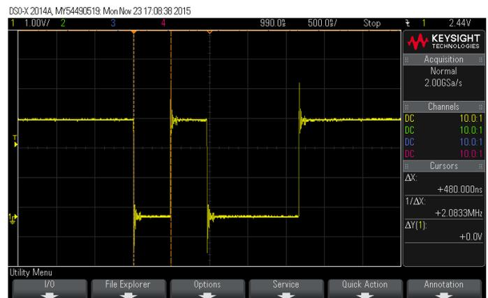
$t_{CD}$  is measured as 1200.0ns.
