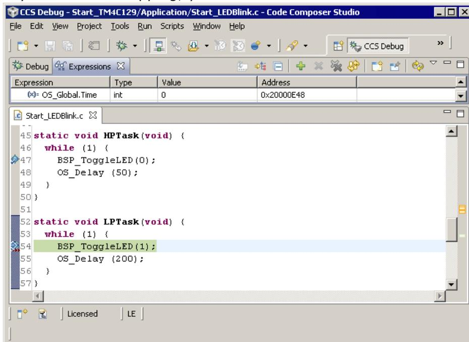
Continue to step through the program, there is no other task ready for execution. embOS will therefore start the idle-loop, which is an endless loop always executed if there is nothing else to do (no task is ready, no interrupt routine or timer executing).
